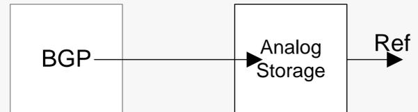
If the chip is in a low power mode the band gap can be switched off but the voltage reference is still available.
